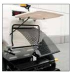
Slide-Out Screen provides easy removal of screen for cleaning.
