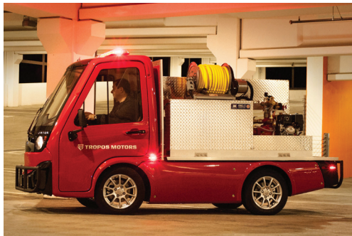
The FRV bed package can transport up to 125 gallons of water.
