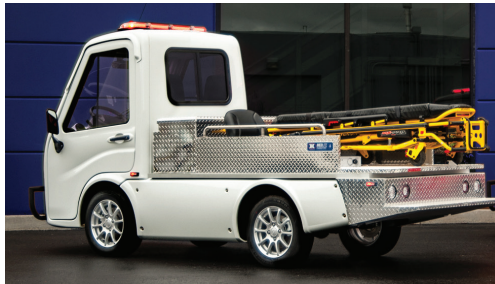
The EMSo bed package offers space for a full-size stretcher, one attendant, and lockable storage
