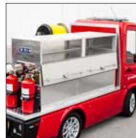
Large hose storage area
