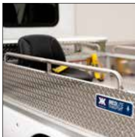
Attendant (and patient) stainless steel grab bars (one on each side of vehicle)
